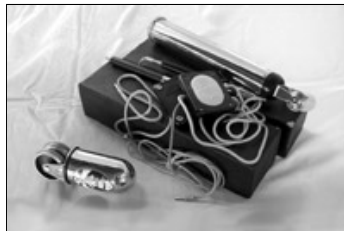
The "Elec-Treat Mechanical Heart" is a battery operated device that produces a mild electrical current for "relief of pain and muscular soreness." The smaller "Magneto Massage Juventude" is rolled over the skin to produce a massage and mild electric shock.
