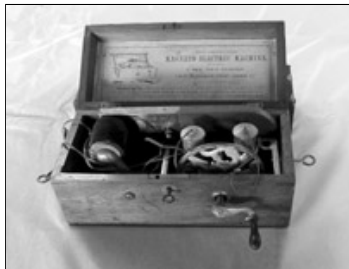
The "Magneto Electric Machine" has a generator powered by turning the handle; it produces a mild electric current as a therapy for many disorders.
